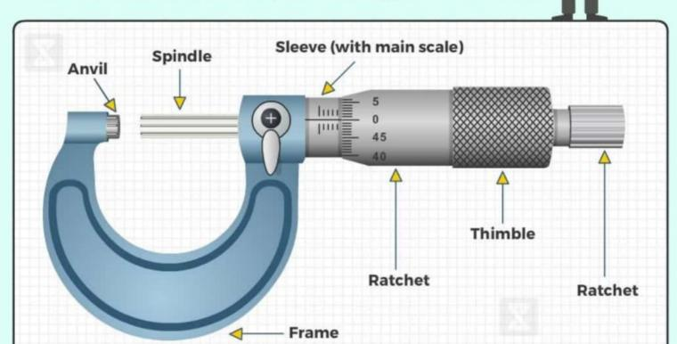
**Pitch:** The pitch of the instrument is distance between two consecutive threads of the screw which is equal to the distance moved by the screw due to one complete rotation of the cap. Thus for,
