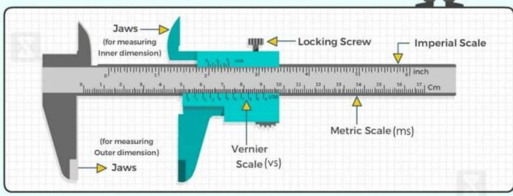
Vernier Constant = 1 ms - 1 vs =  $\left(1 - \frac{N-1}{N}\right)$  ms =  $\frac{1}{N}$ ms, which is equal to the value of the
